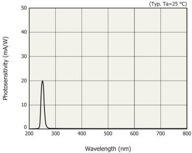
Note: Wavelengths other than 254 nm will be provided on a made to order basis.
