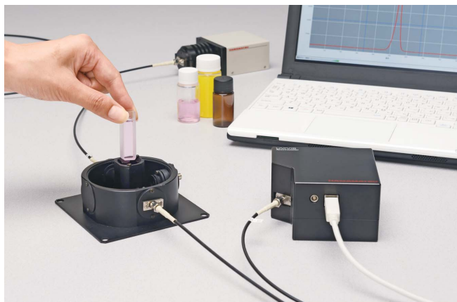
[Figure 26] Connection example (measurement of liquid absorbance)
