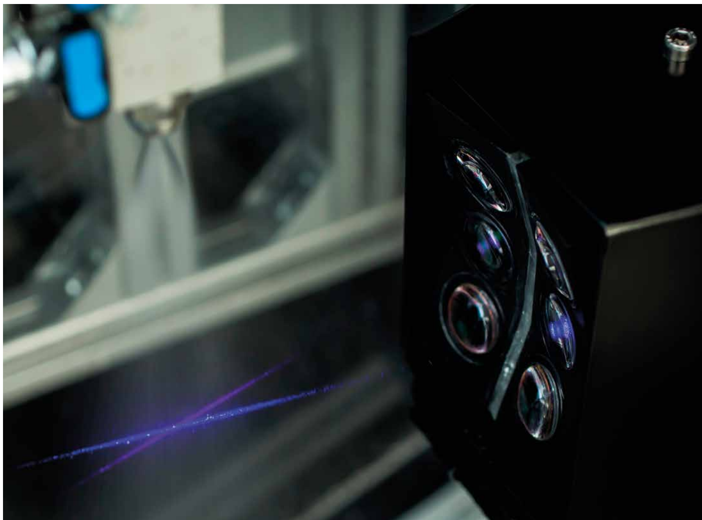
Figure 3: The SpraySpy® measurement system measuring the spray cone of a typical food industry nozzle.
